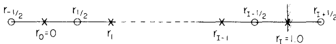
FIG. 1. The radial mesh is extended half a cell beyond the origin ( r = 0 ) and the conducting wall ( r = 1 ).
